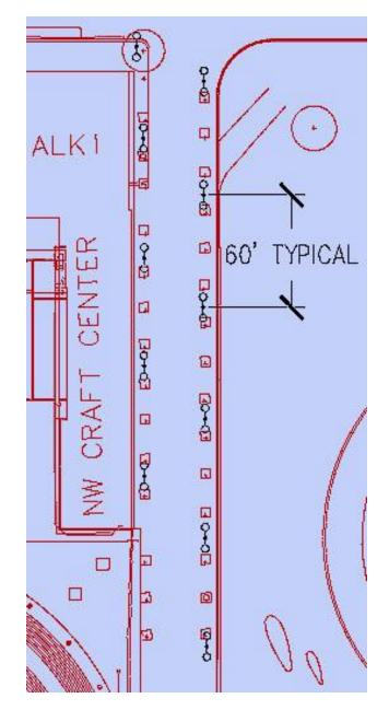
Figure 6: Typical pole layout and spacing for Option 2.
