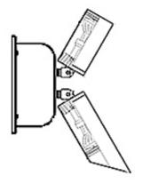
Figure 10: Double headed accent fixtures, with one head directed up to illuminate the canopy, and one directed at the pathway can provide the required functionality without the glare. The uplight component requires a wide spread distribution, probably with the use of a spread lens or reflector, and the downlight component requires source shielding to meet the criteria.
