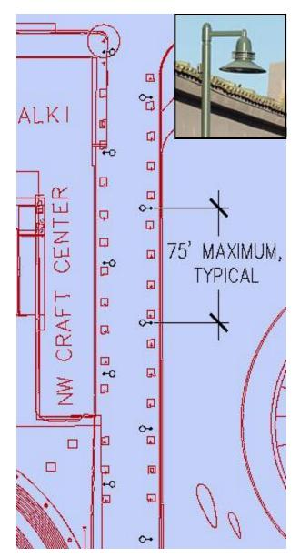
Figure 5: Typical pole layout and spacing for Option 1. Also shown is and example of a typical new proposed pedestrian post-top fixture.
